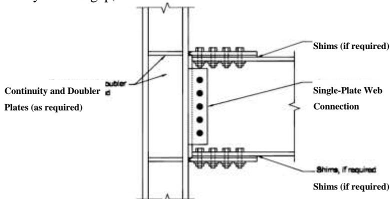
Fig 2. Schematic view of the WUF-B used in the IMRF Structures
