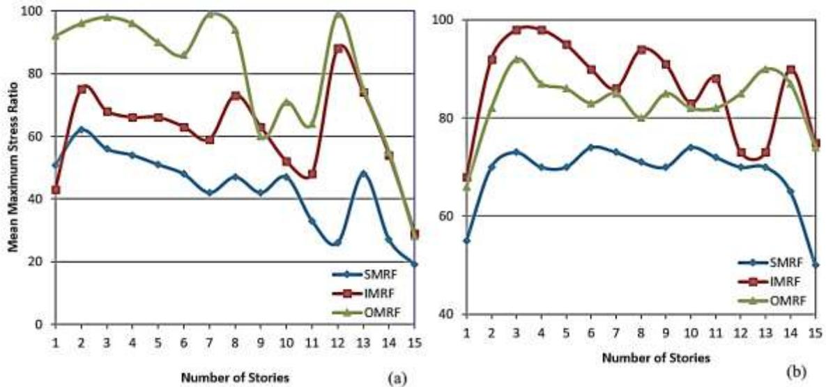
Fig. 9. Mean maximum stress ratios of 9-story structure with five 6-meter bays: (a) Columns, (b) Beams
