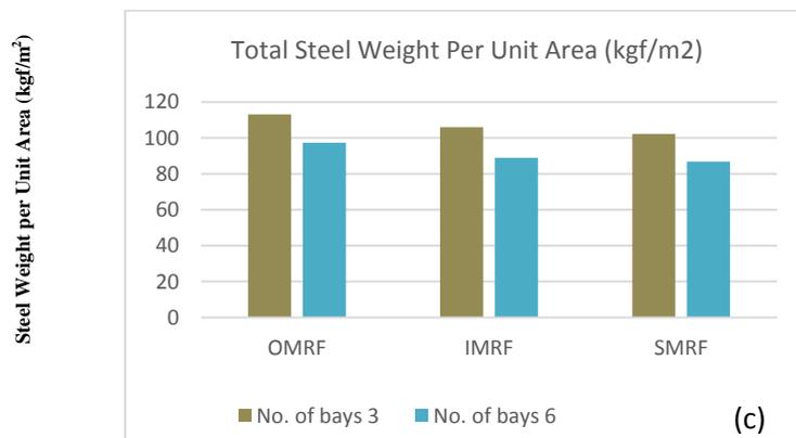
Fig.5. Required steel material weight versus number of bays, (c) The total amount (i.e. beams, columns and connections)
