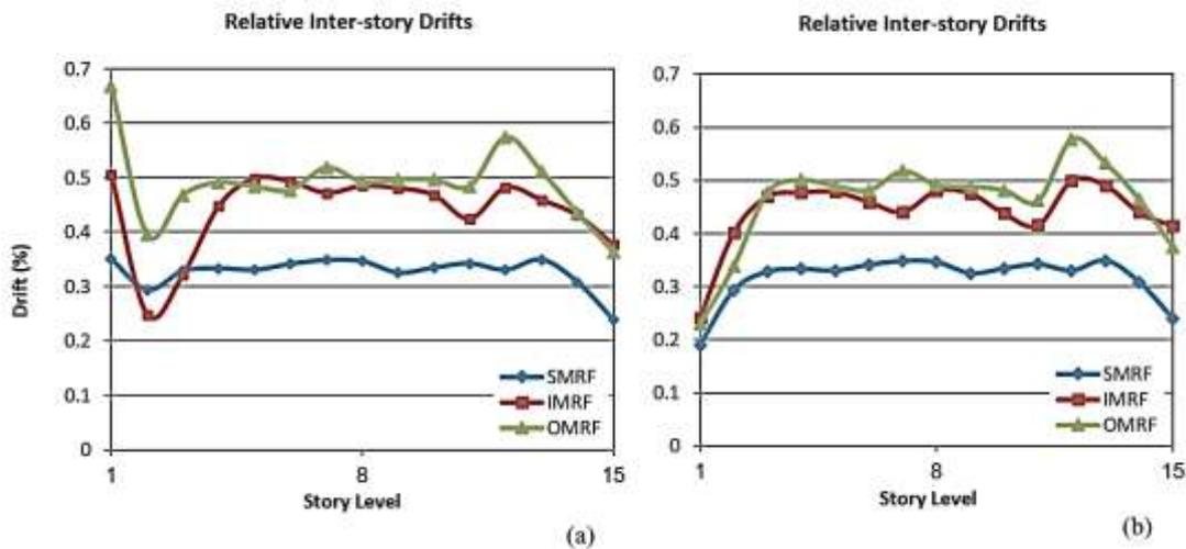
Fig.7. Story drifts of regular structures with six bays and 5-meter spans, (a) No braces, (b) Bottom stories braced
