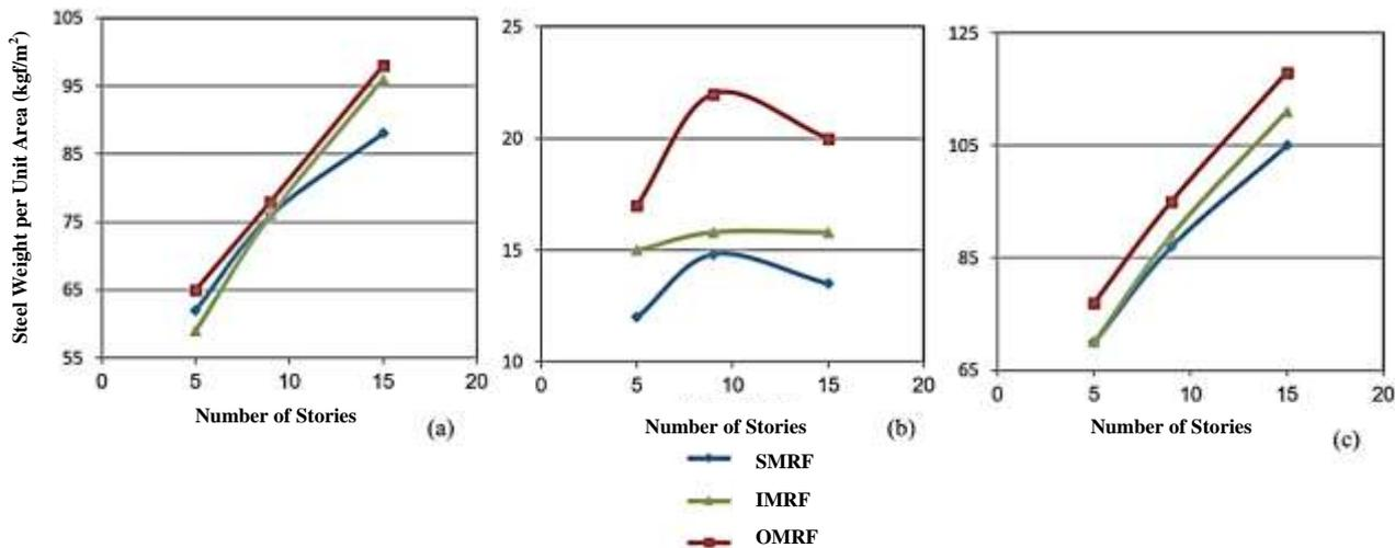
Fig.4. Median steel weight per unit area versus number of stories for SMRFs, IMRFs and OMRFs for (a) Beams and columns, (b) Connections (c) The total amount (i.e. beams, columns and connections)
