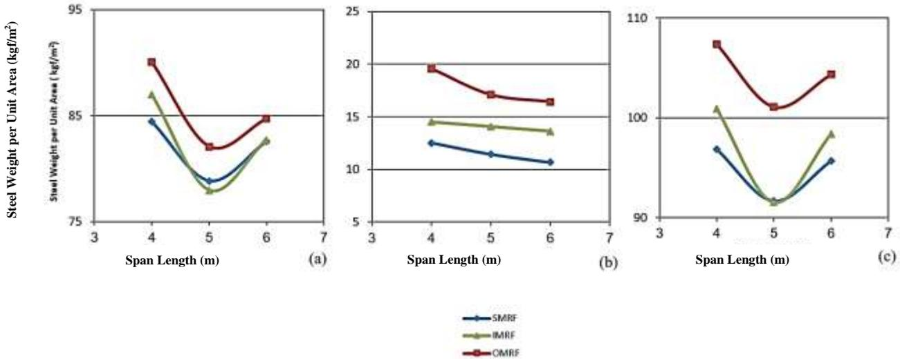
Fig. 6. Required steel material weight versus span length, (a) Beams and columns, (b) Connections, (c) The total amount (i.e. beams, columns and connections)
