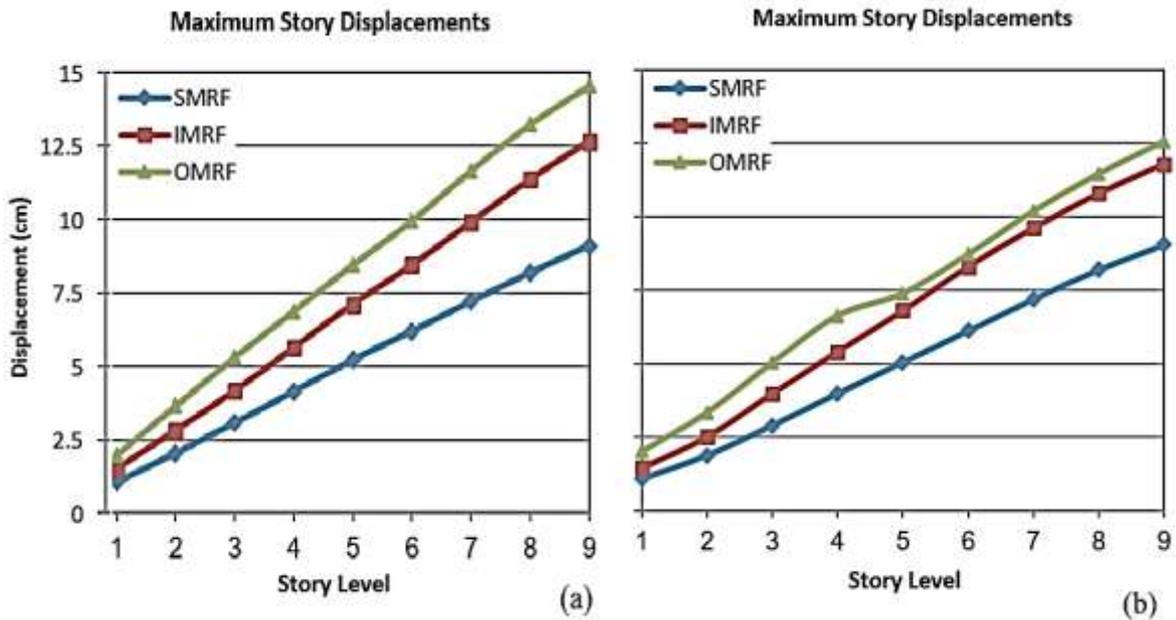
Fig 8. Maximum story displacements of 9-story structures with 5 bays (a) Uniform spans, (b) Non-uniform spans
