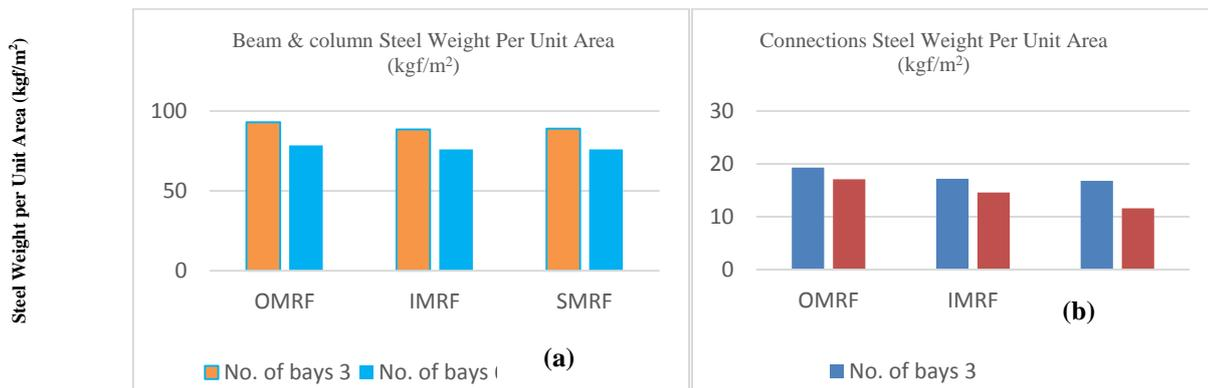
Fig.5. Required steel material weight versus number of bays (a) Beams and columns, (b) Connections
