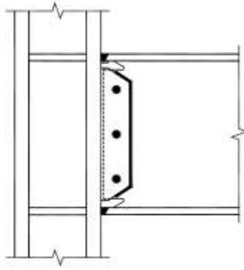
Fig.3. WUF-W connection used in the OMRF Structures
