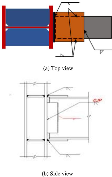
Fig. 1. Schematic View of the used WFP Connection
