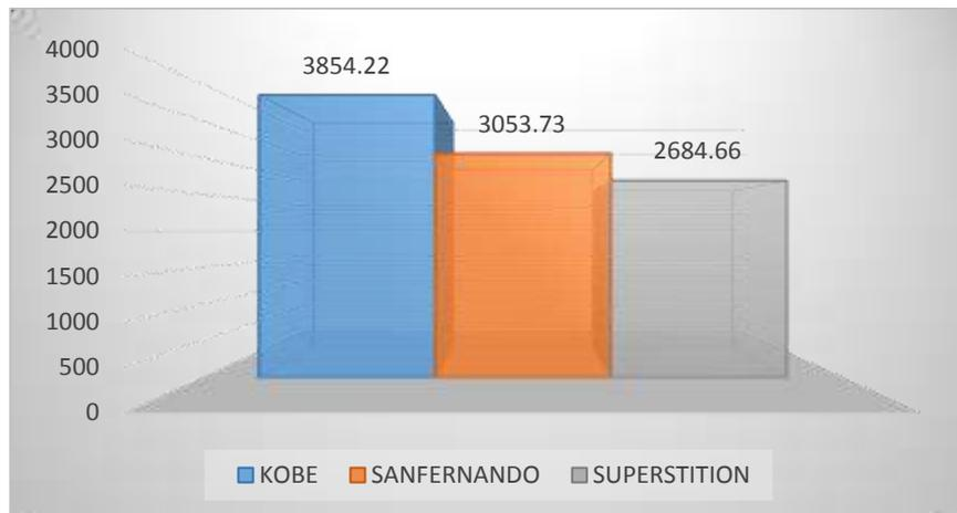
Fig.27. Maximum Torsional Moment Deck Due to Records (KN.m).
