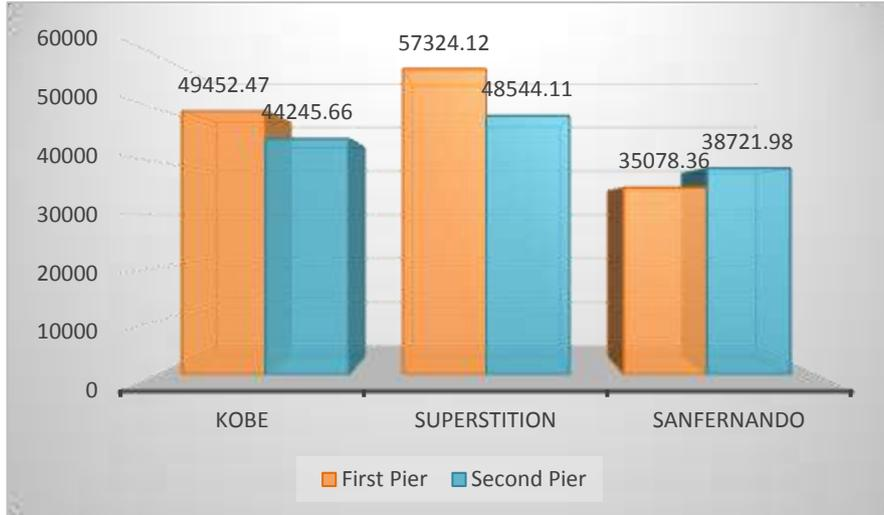
Fig.26. Maximum Axial Force of Bridge Piers Due to Records (KN)
