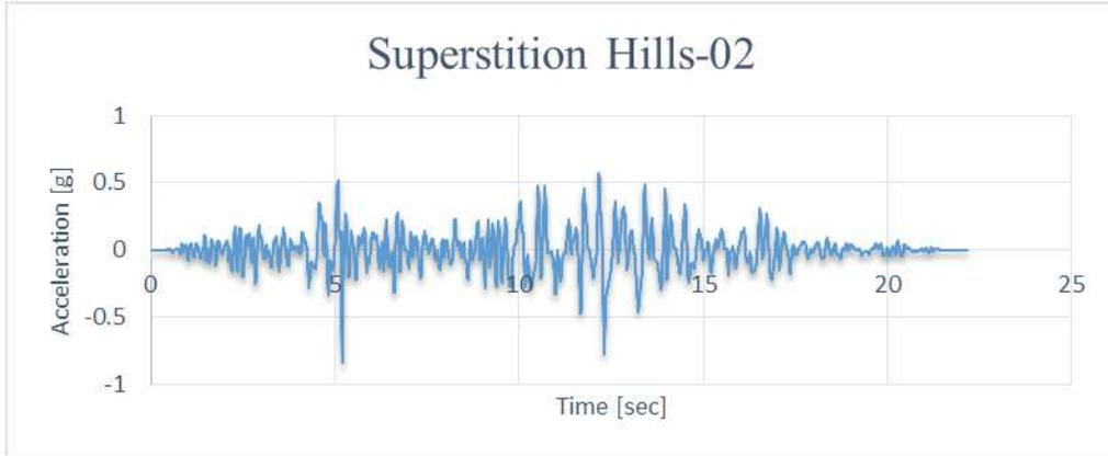
Fig.21. Earthquake Acceleration Applied Superstition to the Structure
