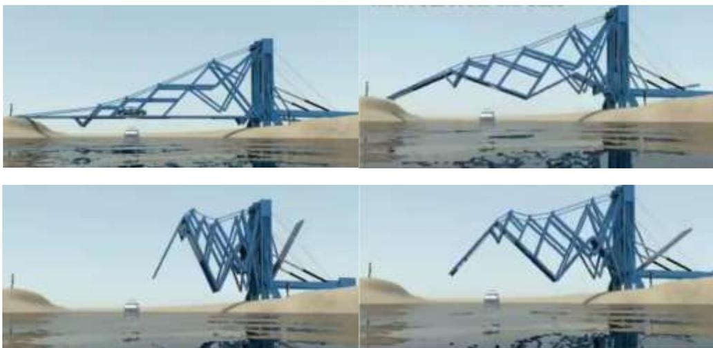
Fig.14. Operation of the Bridge
