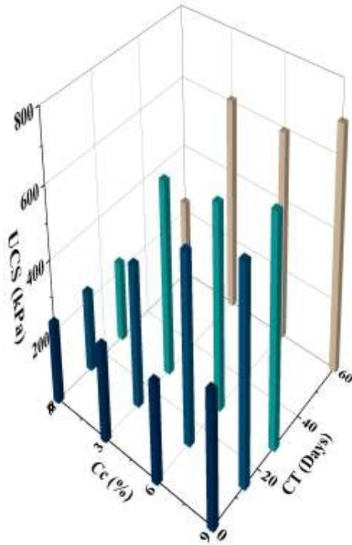
Fig. 6 UCS results of the cement-stabilized specimens at various cement content and curing time.
