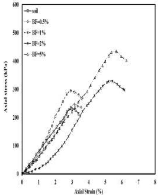
Fig. 8. Stress–strain curves of the BF-reinforced specimens.
