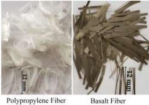
Fig. 3. Photograph showing the discrete short PPF and BF.
