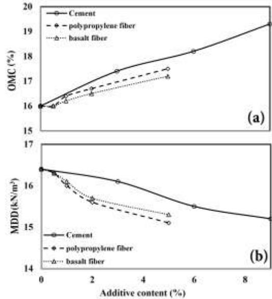
Fig. 4. Variation of OMC and MDD as a function of additive content.
