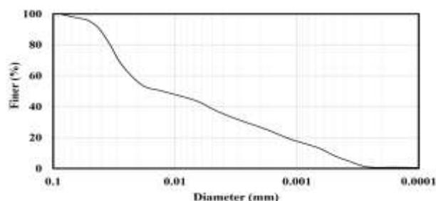
Fig. 1. Grain size distribution curve of the soil
