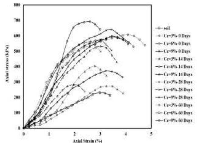
Fig. 5. Stress–strain curves of the cement-stabilized specimens at various cement content and curing time.
