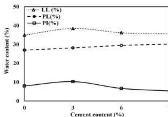
Fig. 2. Variation of LL, PL and PI as a function of cement content.
