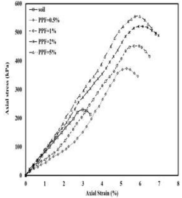
Fig. 7. Stress–strain curves of the PPF-reinforced specimens.
