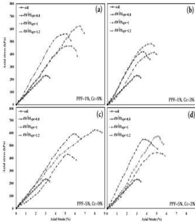
Fig. 9. Stress–strain curves of the PPF-cement-stabilized specimens.
