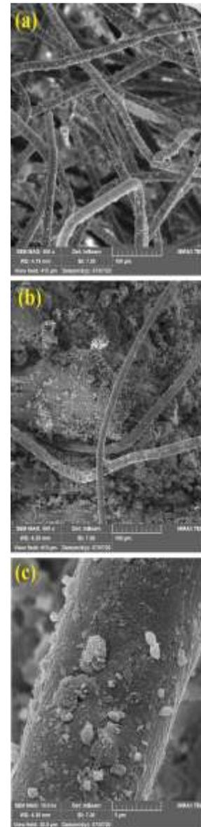
Fig. 12. SEM images of (a) PPF-reinforced specimens (b) PPF-cement-stabilized specimens (c) pits and grooves formed on the PPF surface
