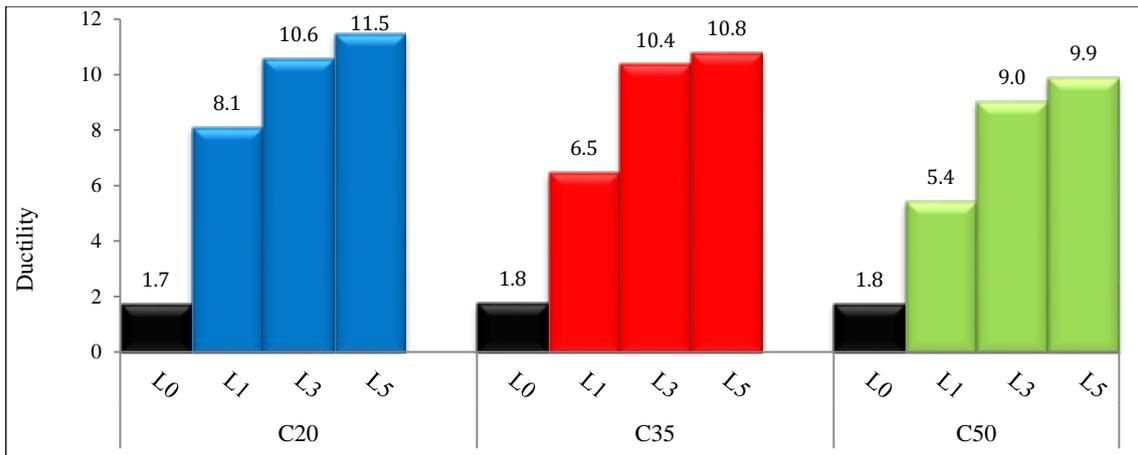
Fig. 7. Ductility of cylindrical samples
