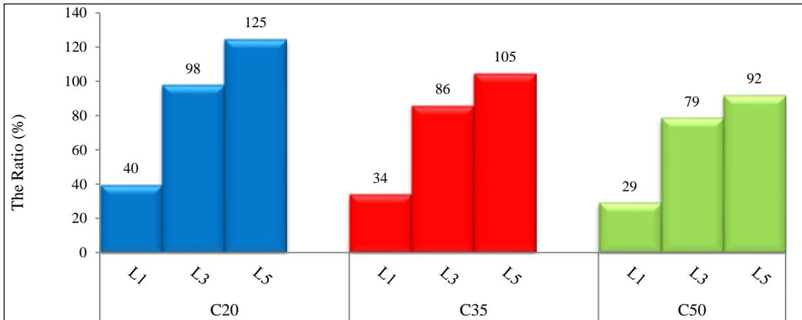
Fig. 6. The ratio of the increase in the compressive strength of samples with increasing number of CFRP layers relative to samples without CFRP
