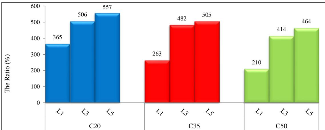
Fig. 8. The ratio of the Ductility of CFRP strengthened samples regarding to non-strengthened samples (%)
