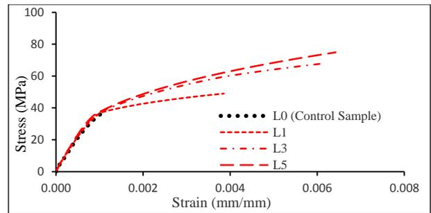
Fig. 3. Stress-strain diagrams for C35 classes
