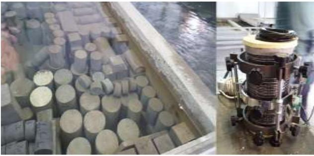
Fig. 1. Samples preparation for stress-strain tests
