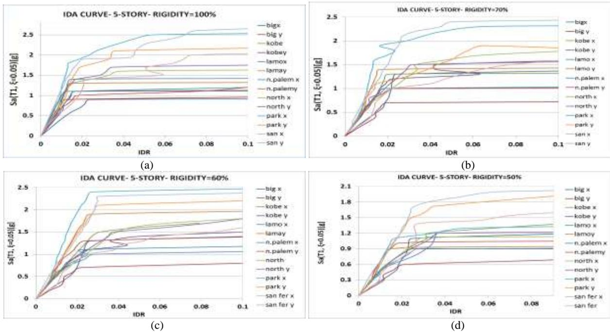
Fig 2. IDA curves of the 5-story frame in four states: (a) Rigid connections, (b) Semi-rigid connections (70% rigidity), (c) Semi-rigid connections (60% rigidity), (d) Semi-rigid connections (50% rigidity)
