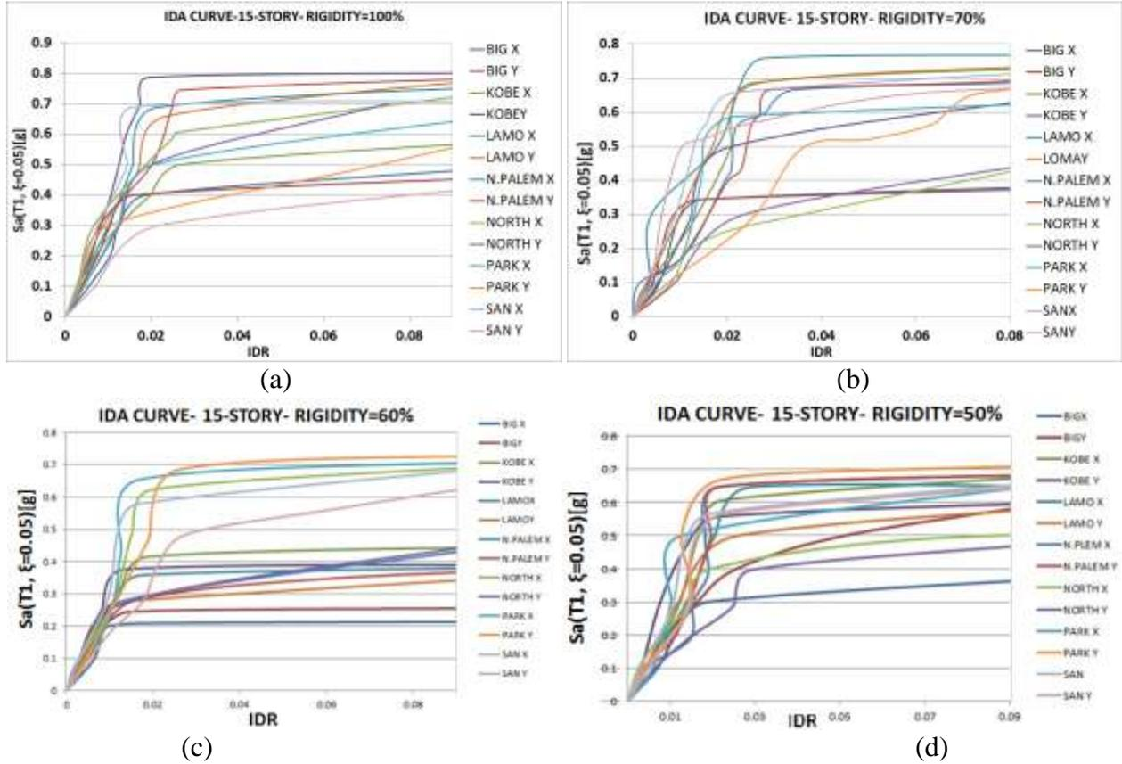
Fig 4. IDA curves of the 15-story frame in four states: (a) Rigid connections, (b) Semi-rigid connections (70% rigidity), (c) Semi-rigid connections (60% rigidity), (d) Semi-rigid connections (50% rigidity)
