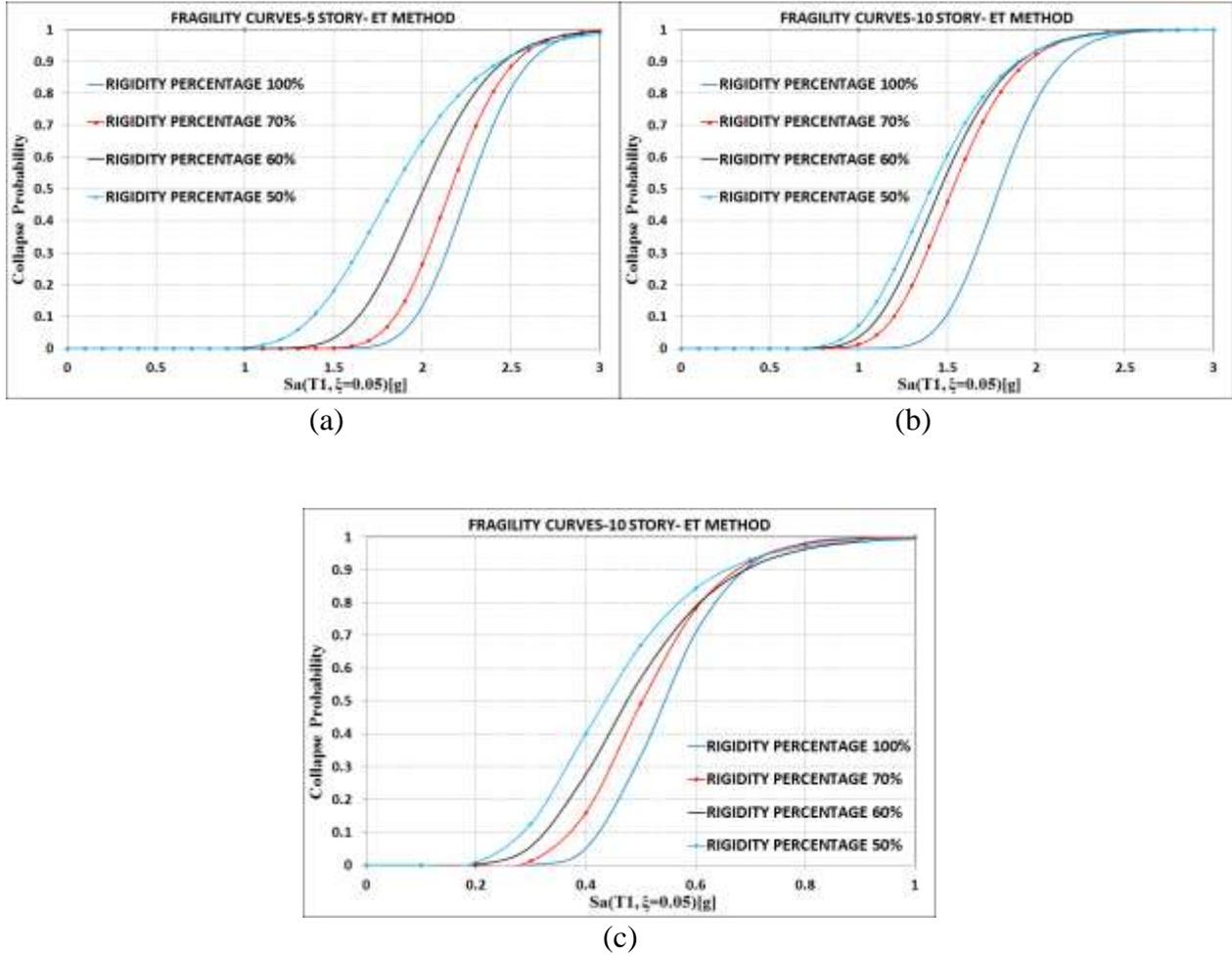
Fig 7: Fragility curves of the studied frames obtained using the ET method in different rigidity percentage: (a) 5-story frame, (b) 10-story frame and (c) 15-story frame
