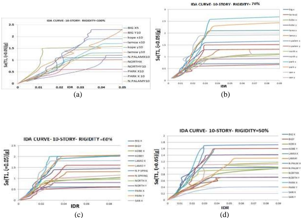
Fig 3. IDA curves of the 10-story frame in four states: (a) Rigid connections, (b) Semi-rigid connections (70% rigidity), (c) Semi-rigid connections (60% rigidity), (d) Semi-rigid connections (50% rigidity)
