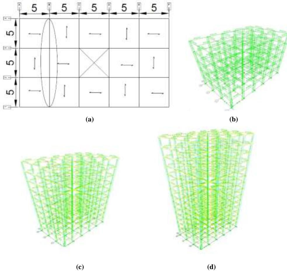
Fig. 1. Structural plan, elevation and selected frame
