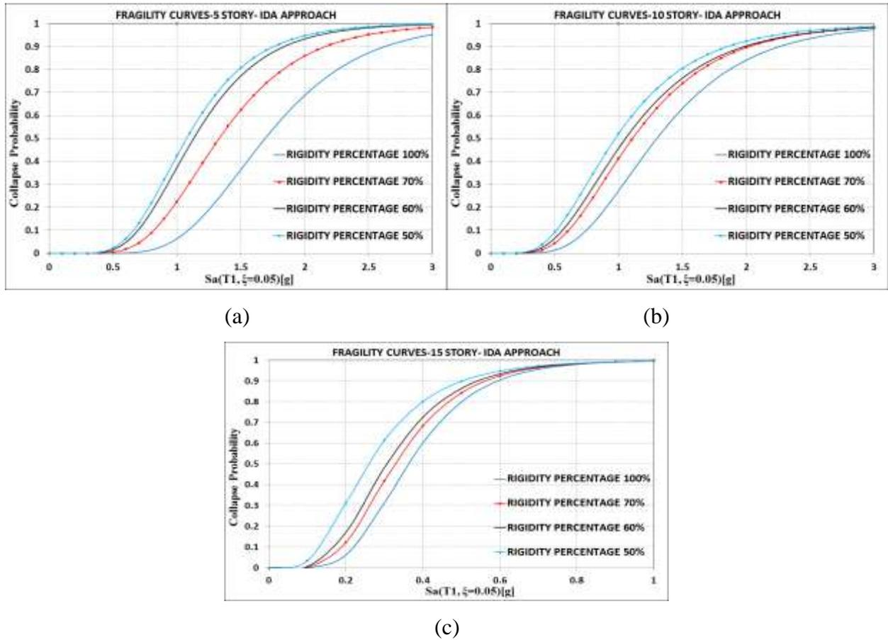
Fig 1: Fragility curves of the studied frames obtained using the IDA method in different rigidity percentage of connections: (a) 5-story frame, (b) 10-story frame and (c) 15-story frame
